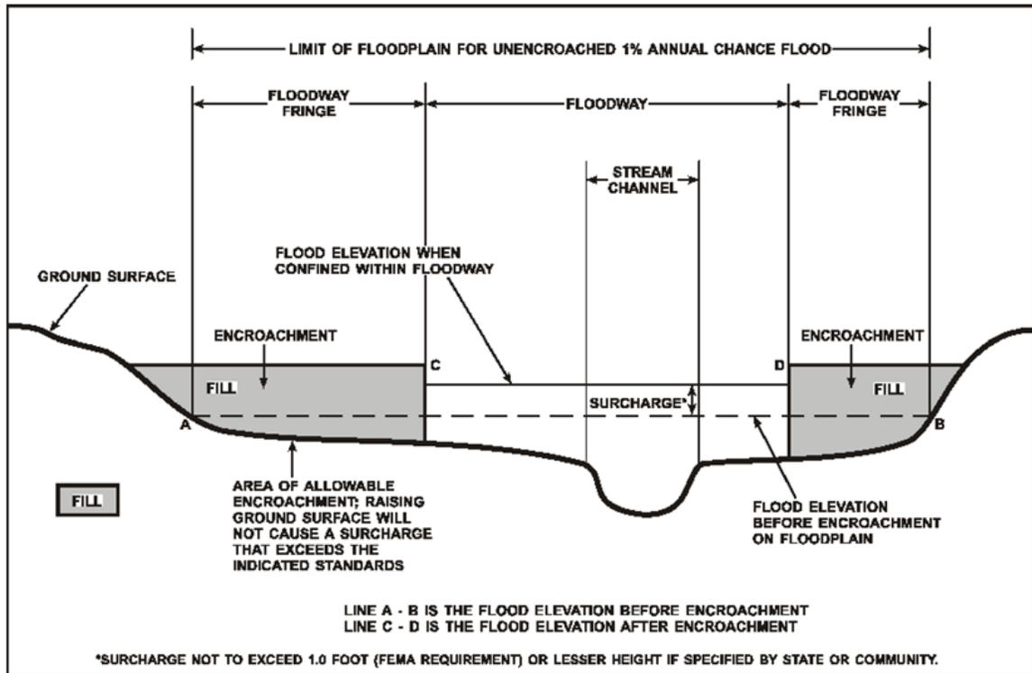
Floodway widths presented in this FIS Report and on the FIRM were computed at cross sections. Between cross sections, the floodway boundaries were interpolated. For certain stream segments, floodways were adjusted so that the amount of floodwaters conveyed on each side of the floodplain would be reduced equally. The results of the floodway computations have been tabulated for selected cross sections and are shown in Table 23, "Floodway Data."
